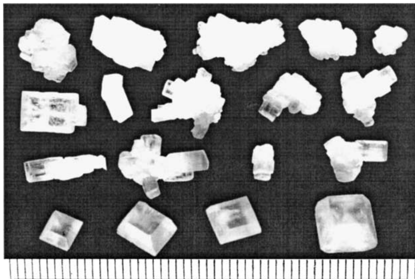
Figure 2 Different morphologies of calcium malonate hydrate crystals grown by the gel-aided solution technique.
